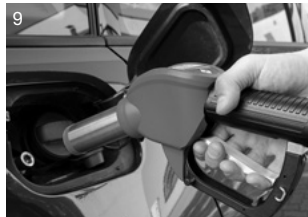
Remove nozzle and put back in dispenser nozzle holder.
