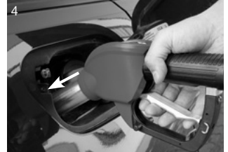
Push nozzle firmly onto the vehicle filling point.
