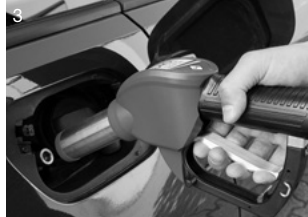
Take nozzle from dispenser. Align nozzle with vehicle sided fill point as shown.
