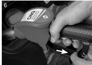
Hold the lever pulled and lock the hold-open latch as shown to open the nozzle valve. Release the lever and it will stay in the open position. Do not lean on / tilt the nozzle.
