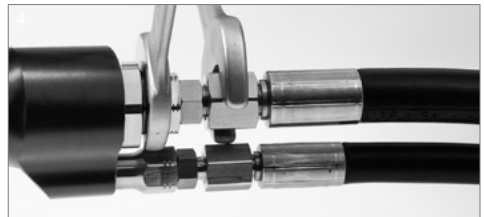
Connect the hoses to the nozzle. Torque the fill line to 45 Nm and torque the vent line to 35 Nm or as per hose fitting suppliers recommended tightening torque. Do not use pliers.
