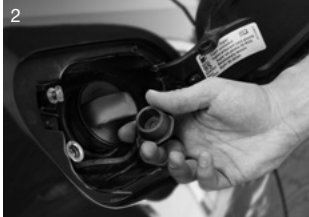
Ensure that all coupling parts, seals and sealing surfaces of nozzle and vehicle filling point are clean and undamaged.
