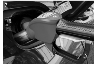
Fuelling should start automatically OR has to be activated at the dispenser. Please follow operating instructions displayed at the dispenser.
