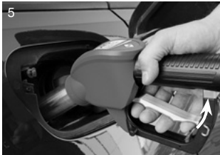
In that position, pull the lever. If the nozzle is correctly coupled, a green indicator ring appears on the coupling part — from the nozzle side.
