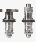
Protects LNG dispensers from drive-away incidents by separating and isolating dispenser from Fill or Vent Line. Stops the flow of fuel on both ends at separation. Reconnectable after breakaway event by replacing breaking bolts EB 544-3. For installation on LNG dispensers.
