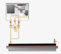
SGB leak detectors realize highest environmental protection according to EN 13160 (class I) for double-walled pipes: Both inner and outer wall are monitored 100% continuously and reliably for leaks. Loss of the conveyed product is excluded due to the pneumatic monitoring principle.
