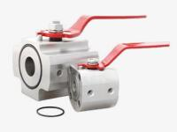
Quarter turn manual cylinder ball valve designed for fast load/unload of gas cylinders. Mainly used in CNG applications where time and safety are critical factors. Full flow 1/2" for cylinder threads 1 1/8-12 UNF. Other options on request.
